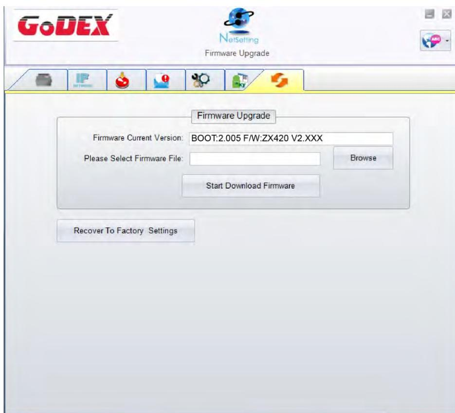
In addition to the firmware update, you can press “Recover To Factory Settings” button to restore the printer configurations back to factory default.
