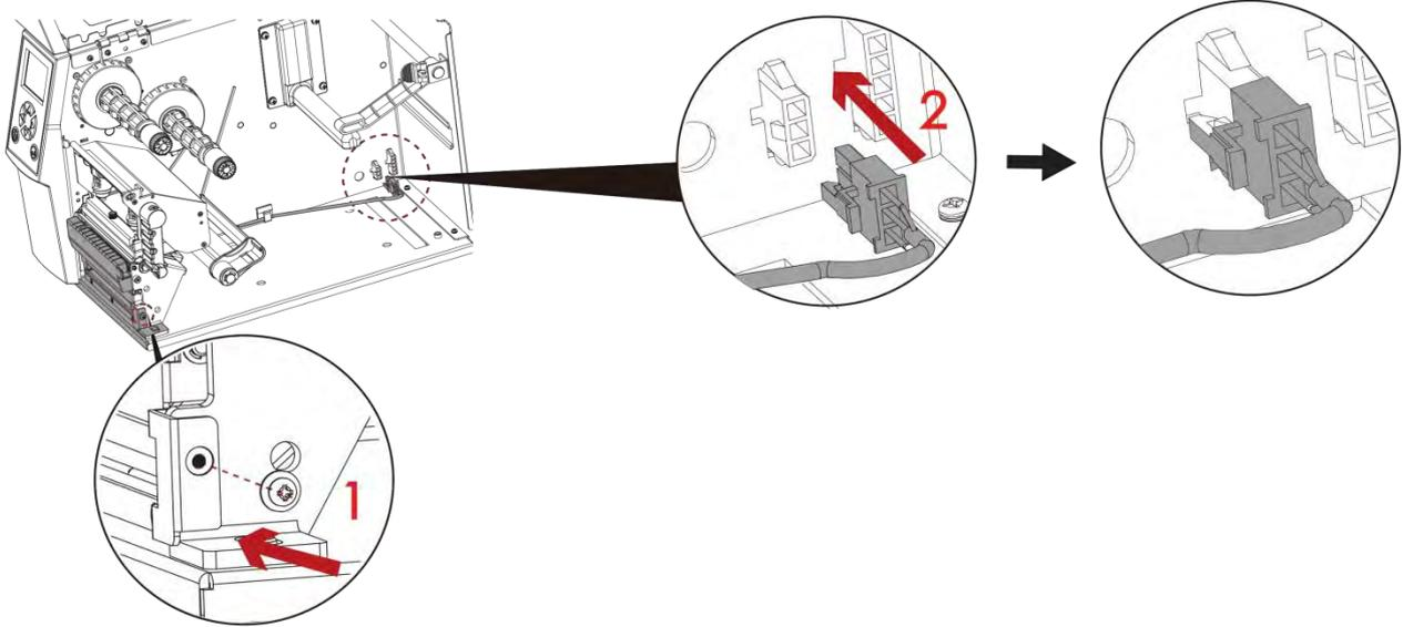
7. Put the cable into the hub.
