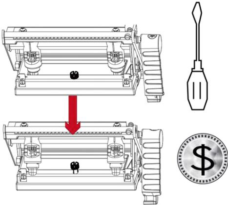
2. Using a screwdriver or a coin to loosen the screw to loosen the screw
