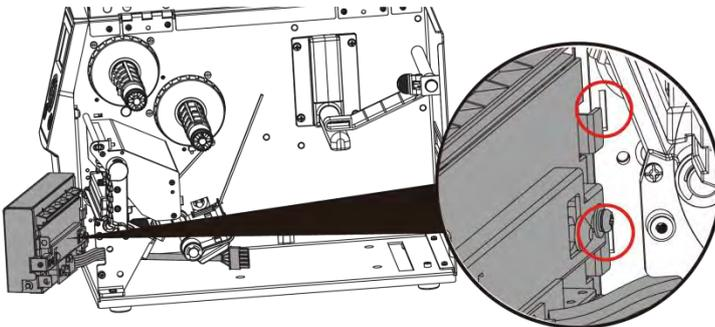
5. Engage the catches of the cutter module firmly into the printer.
