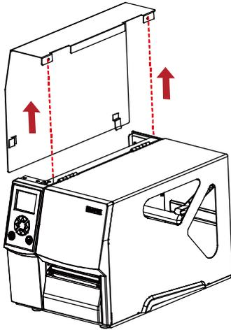
Step2. Disassemble the left side cover.
