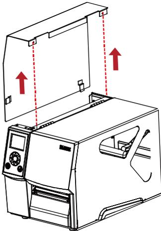
Step2. Disassemble the left side cover.
