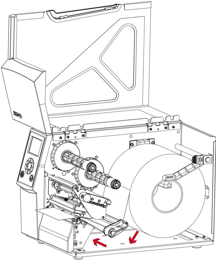
**Load the label roll into the printer as shown in the illustration.
