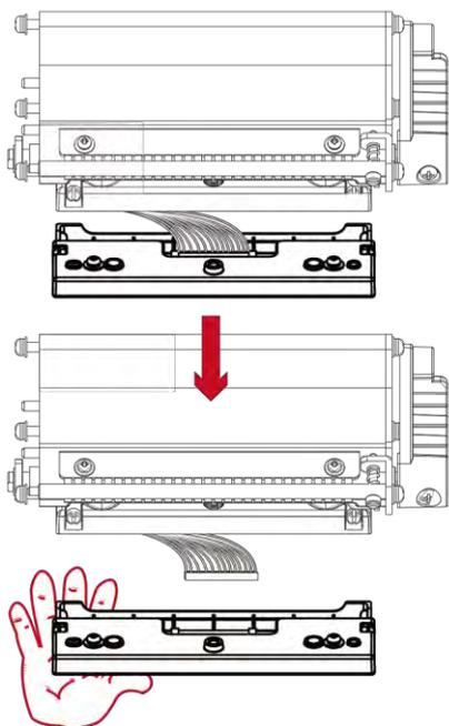
2. Using a screwdriver or a coin, loosen the screw to take out the TPH module.
