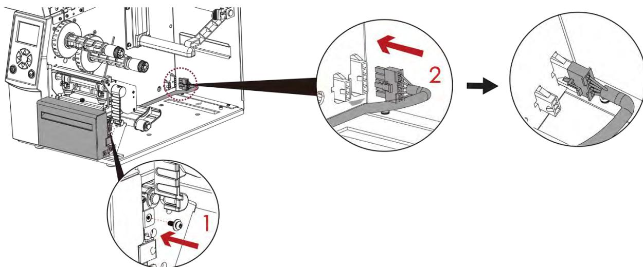
7. Put the cable into the hub.
