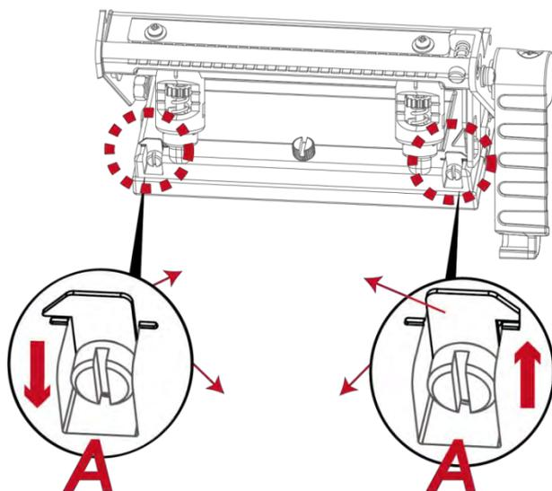
If no improvement is visible, turn the screws(A) clockwise or counterclockwise as far as possible and be sure to align with the indicator board and indicator line. Repeat the adjustment process until printing quality has improved.
