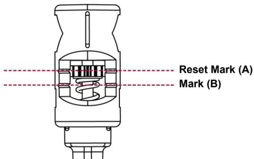
Turning the screw left increases the pressure,
