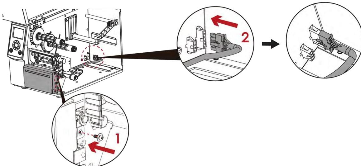
7. Put the cable into the hub.
