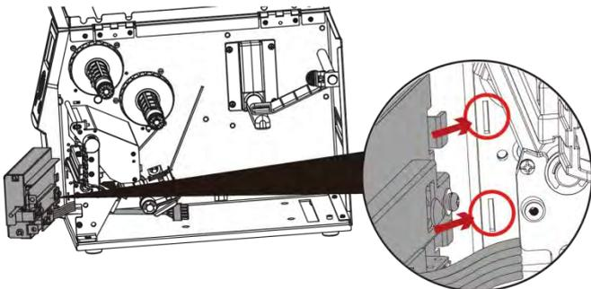
5. Engage the catches of the cutter module firmly into the printer.
