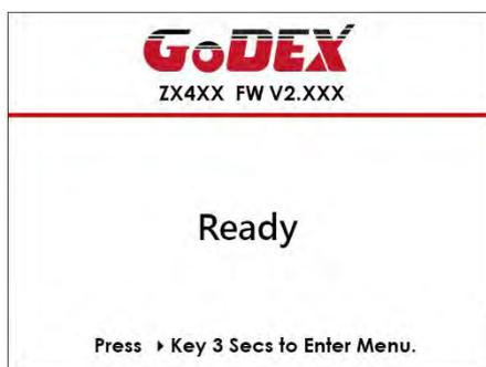
Please keep pressing ▶ button and wait for the timer to be filled, then the LCD interface will enter into the MAIN PAGE for SETTING MODE. You can make various setting functions in SETTING
