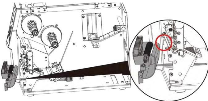
5. Engage the catches of the label dispenser module firmly into the printer.
