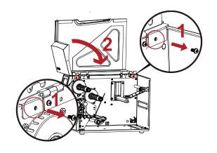
Step1. Remove the screw on the left side cover.
