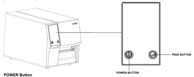
Press the POWER button to turn on the printer, and the START UP SCREEN appears. The printer is on "ready to print" status. When printer is turned on, hold and press down the POWER button for 3 second will turn the printer off.
