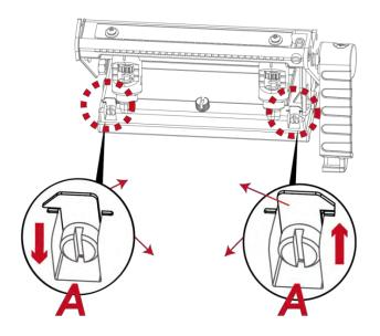
If no improvement is visible, turn the screws(A) clockwise or counterclockwise as far as possible and be sure to align with the indicator board and indicator line.
