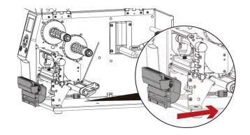
4. Direct the label dispenser's cable through the platen bracket of the printer.
