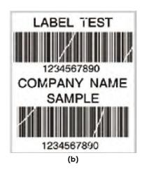
To keep track of the change in print quality, you should adjust the screws by half a turn at a time. Print a test page. If there is no improvement in the print result, turn the screw by another half turn. Do not turn the adjustment screw more than two full turns (360°).
