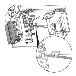
7. Put the cable into the hub.
