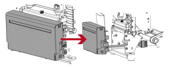
Switch off the printer before removing the CUTTER.
