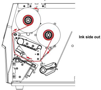
Pass the ribbon under the print head and back up on the other side.
