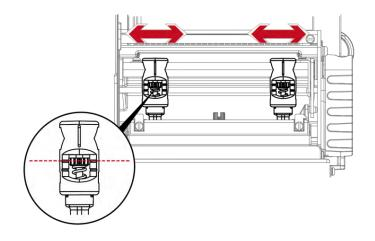
Turning the screw left increases the pressure,
