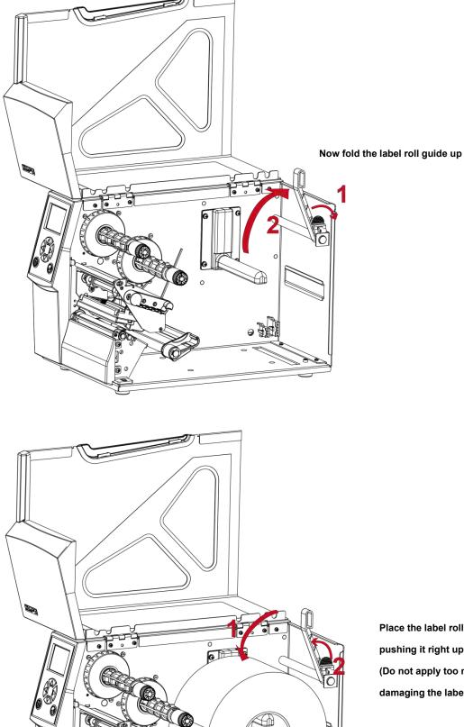
Place the label roll on the label supply hub, pushing it right up to the printer housing.
