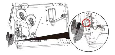
5. Engage the catchs of the label dispenser module firmly into the printer.
