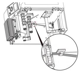
7. Put the cable into the hub.
