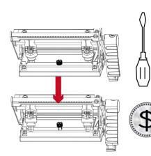
Using a screwdriver or a coin, loosen the screw to take out the TPH module.
