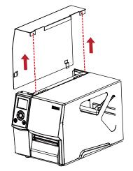
Step2.Disassemble the left side cover.
