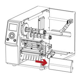
2. Remove the cover panel by pushing to right-hand side.
