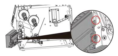
5. Engage the catchs of the cutter module firmly into the printer.
