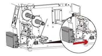
4. Direct the cutter's cable through the platen bracket of the printer.
