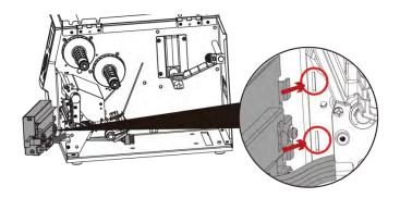
5. Engage the catchs of the cutter module firmly into the printer.
